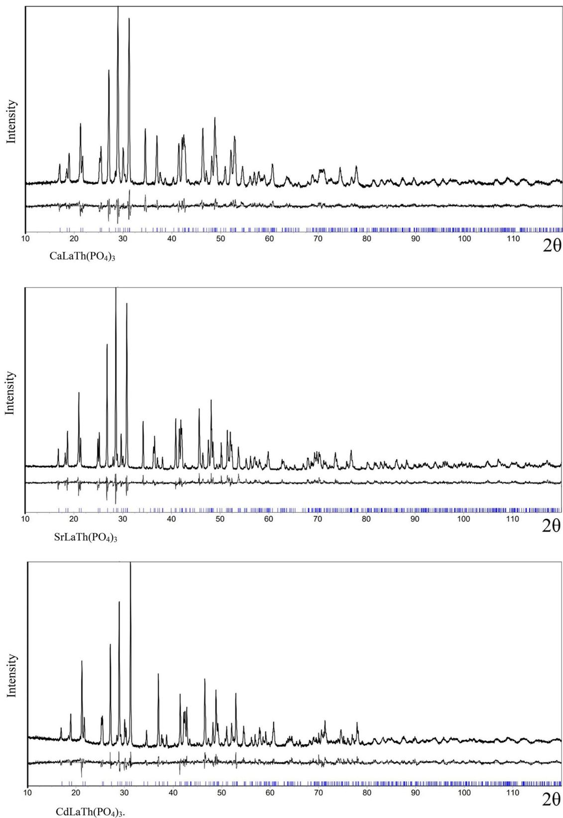
**Fig. 1** The calculated, experimental profiles (upper curves) and difference X-ray diffraction patterns (bottom curve) for the compounds CaLaTh(PO<sub>4</sub>)<sub>3</sub>, SrLaTh(PO<sub>4</sub>)<sub>3</sub>, CdLaTh(PO<sub>4</sub>)<sub>3</sub>. Reflection positions are presented by vertical hash marks
