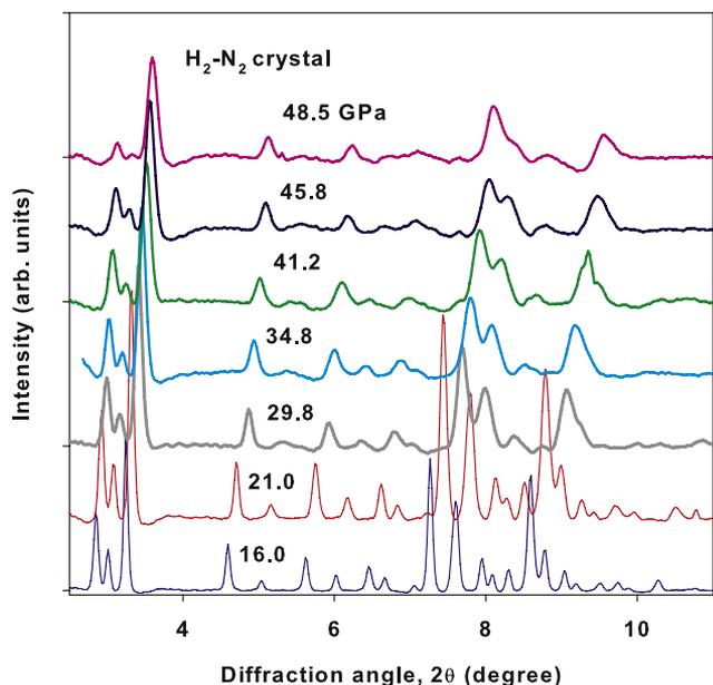
FIG. 3. X-ray diffraction patterns of a  $\text{H}_2\text{-N}_2$  van-der-Waals compound as a function of pressure. The x-ray wavelength was  $0.3344\text{ \AA}$ .
