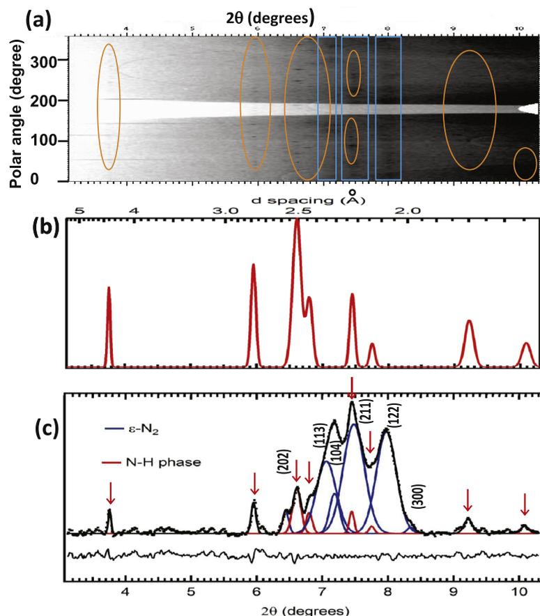
FIG. 8. X-ray diffraction pattern at 55 GPa after the transformation to the oligomeric phase. (a) 2D x-ray diffraction (cake), the ovals, and rectangles show the areas with diffraction of the new phase and molecular nitrogen, respectively; (b) extracted x-ray diffraction of a synthesized phase; (c) the deconvolution of peaks of molecular nitrogen (the main peaks are indexed) and oligomeric phase (marked by red arrows) in the integrated pattern. The x-ray wavelength was 0.2893 Å.
