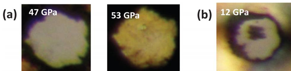
FIG. 2. Transformation of the  $\text{H}_2\text{-N}_2$  van-der-Waals crystal at  $P > 47$  GPa and 11.3 GPa: (a) microphotographs showing a change in color and grain structure; (b) image shows the formation of a new phase (a dark spot) after UV irradiation at 11.3 GPa.
