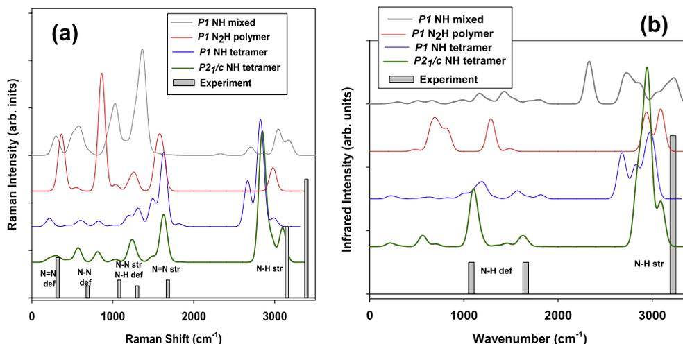
FIG. 11. Theoretically computed at 50 GPa Raman (a) and IR (b) spectra of the most stable hydronitrogens in comparison with the experimental data (at 55 GPa) for the compound synthesized at 47 GPa.
