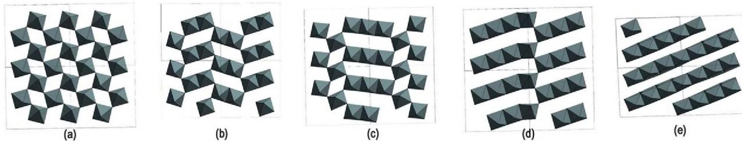
Metadynamics results for compressed MgSiO<sub>3</sub>. Transition from perovskite to post-perovskite is compatible with (ARO et al., Nature 2005).
