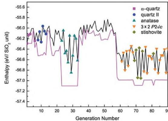
Metadynamics results for compressed SiO<sub>2</sub>. After a disordered state is formed, the system recrystallized!
