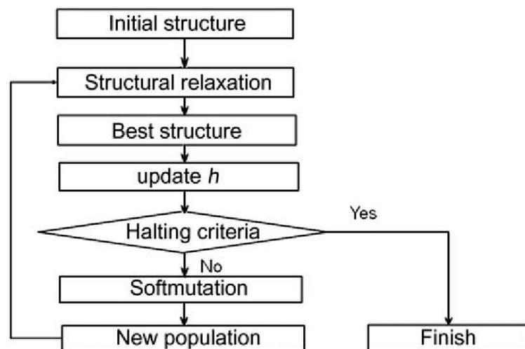
**I. Flowchart of evolutionary metadynamics. The method is evolutionary because in each metastep (generation) there are many structures, and the one with lowest energy (at fixed cell!) is selected to produce offspring.**
