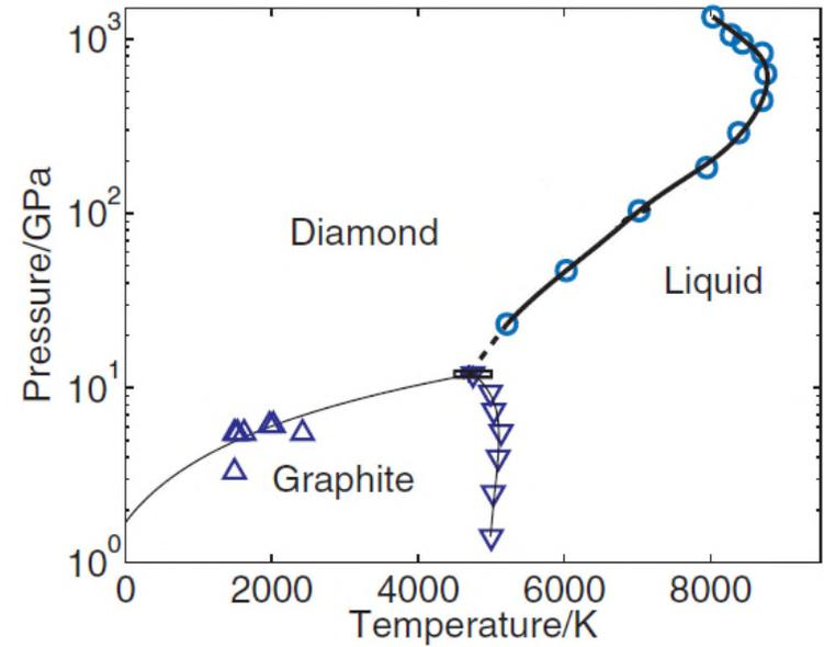
Theoretical phase diagram of carbon [Wang et al. (2005)]
