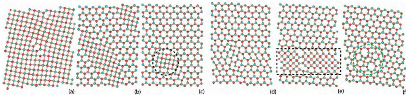
**B1-B4 transition pathway in ZnO [Boulfelfel et al. (2007)]**
