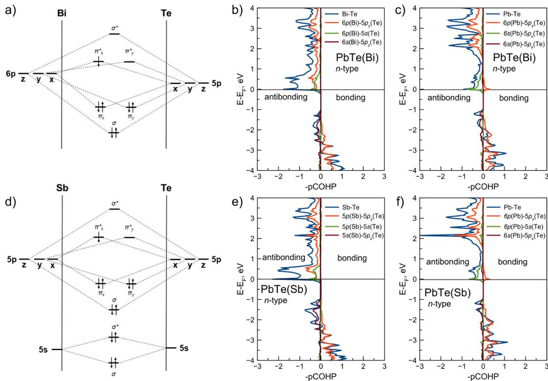
**FIG. 5.** (a) and (d) Electronic structure of the PbTe doped with the  $n$ -type dopant; (b) and (e) COHP diagrams for the interaction between the dopant atom and the nearest Te atom; and (c) and (f) COHP diagrams for the interaction 5 on Fig. 3.
