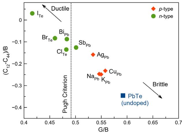
**FIG. 1.** Correlation between  $(C_{12}-C_{44})/B$  and  $G/B$ , where  $B$  is the bulk modulus, and  $G$  is the shear modulus. Top left points correspond to more ductile materials, while bottom right points correspond to more brittle ones. Pugh criterion was calculated for pristine PbTe.
