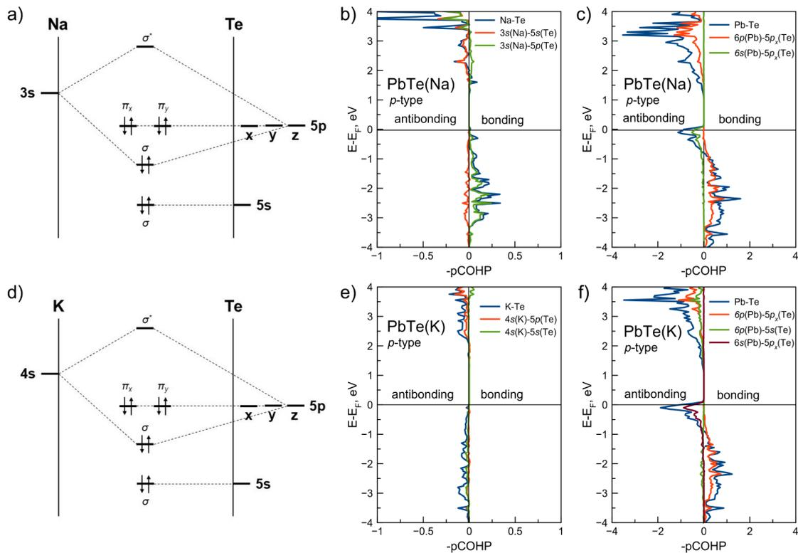
**FIG. 4.** (a) and (d) Electronic structure of the PbTe doped with the  $p$ -type dopant; (b) and (e) COHP diagrams for the interaction 1 between the dopant atom and the nearest Te atom; and (c) and (f) COHP diagrams for the interaction 5 on Fig. 3.
