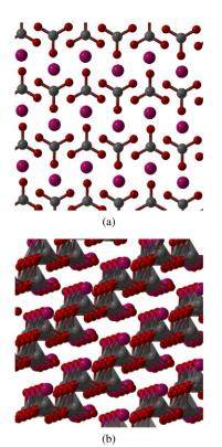
Fig. 5. (a) Post-aragonite phase of  $CaCO_3$  identified by USPEX. (b) Phase I (orthorhombic  $C222_1$ ) identified by USPEX.
