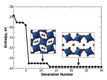
Fig. 4.  $MgSiO_3$  at 120 GPa. Enthalpy of the best individual versus generation. Population size: 30.
